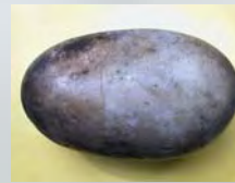
Condition of heating stone after experiment, major fracture lines visible.
