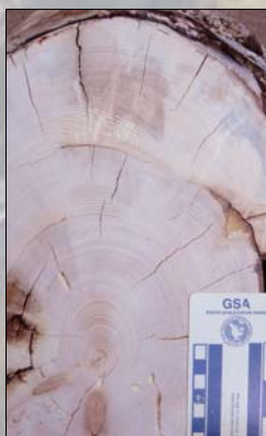
Figure 3: Cross section taken from tree for dendrochronology dating
